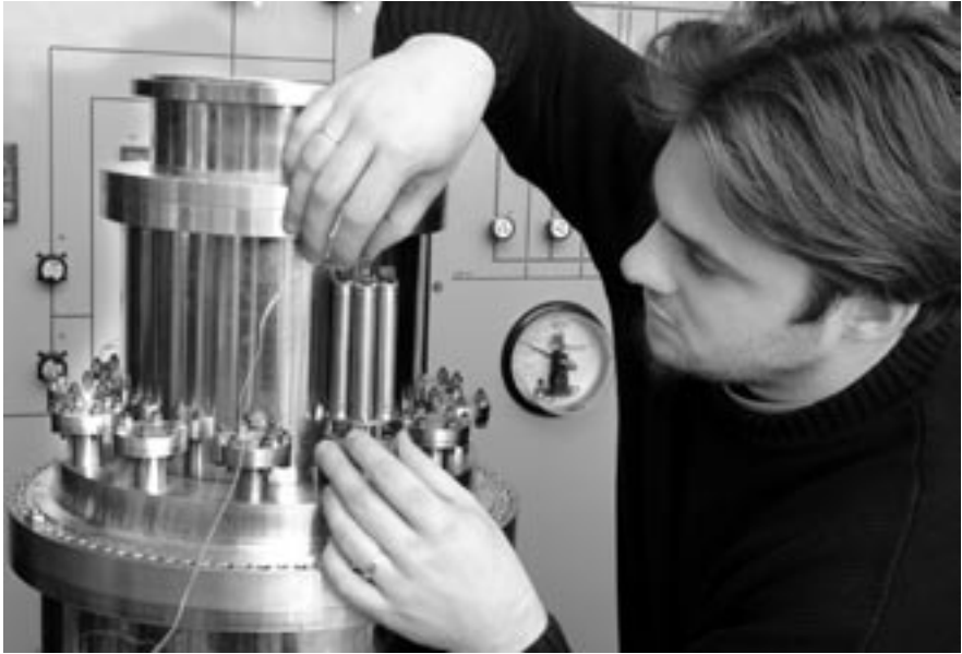
Installation of SQUID sensors for the CRESST dark matter search
