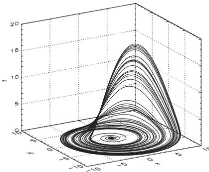
The figure shows an integration of the Rössler system with  $a = b = 0.2$  and  $c = 5$ , with the heavy dot marking the initial conditions close to the more stable fixed point. In this vicinity, show that perturbations in one direction decay rapidly, confining the attractor close to a two-dimensional surface. Discuss the evolution of the trajectory as it moves further away from the fixed point, using your expressions for the growth rate of perturbations to explain how trajectories diverge.
