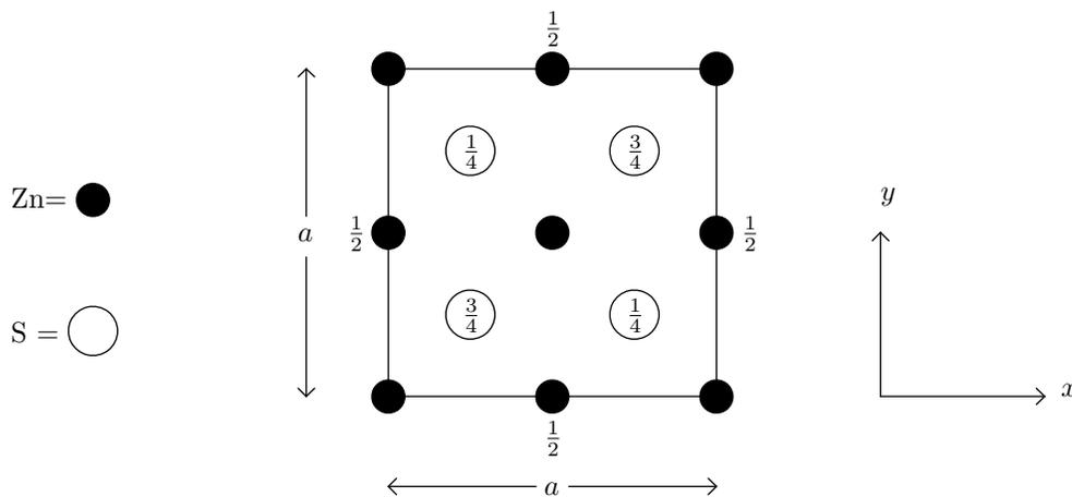
The diagram above shows a plan view of a structure of cubic ZnS (zinc blende) looking down the  $z$  axis. The numbers attached to some atoms represent the heights of the atoms above the  $z = 0$  plane expressed as a fraction of the cube edge  $a$ . Unlabeled atoms are at  $z = 0$  and  $z = a$ .
