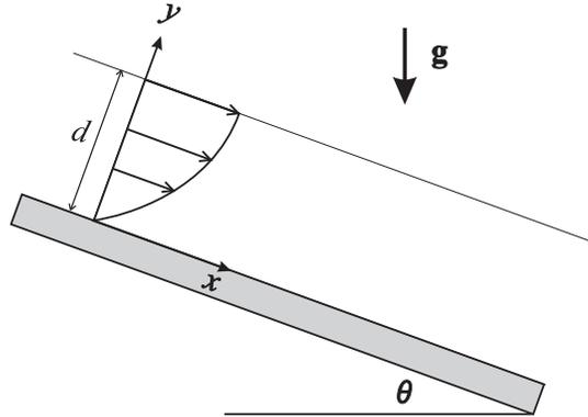
What are the boundary conditions for  $u$  and  $v$  at  $y = 0$ ? Using incompressibility, show that  $v = 0$  throughout the flow. Write down the  $x$ - and  $y$ -components of the Navier-Stokes equation, and from the  $y$ -component show that the pressure is of the form  $p(x, y) = -\rho g y \cos \theta + F(x)$ , where  $F$  is an arbitrary function. Assuming that the pressure at the free surface  $y = d$  equals the constant atmospheric pressure  $p_0$ , show further that
