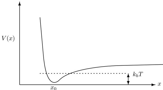
where  $x$  is the distance between the two neighboring atoms. This potential can be expanded around its minimum as
