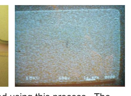
Optical and SEM closeups of a trap and a single DC electrode fabricated using this process. The high aspect-ratio of the insulating gaps shields the ion from the potentially charged substrate.
