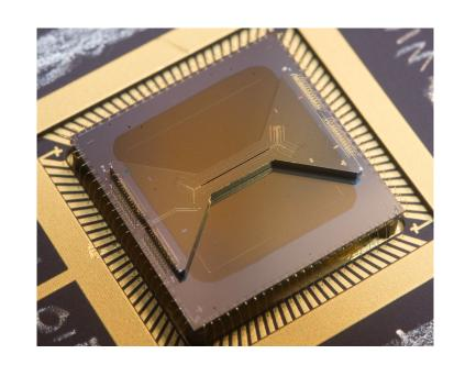
We have constructed two identical vacuum systems, each containing a HOA2 multi-zone surface linear trap (courtesy of Sandia National Labs), designed to operate with both <sup>43</sup>Ca<sup>+</sup> and <sup>88</sup>Sr<sup>+</sup> and allow high-fidelity mixed species gates.
