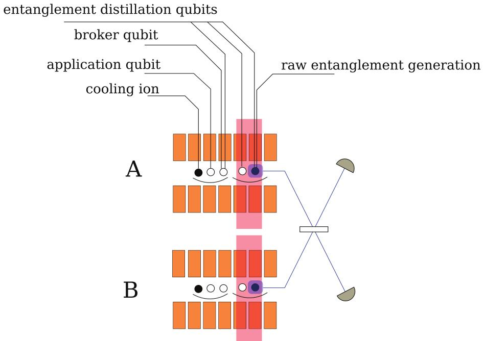
We collect photons perpendicular to the magnetic field - coupling into a single (Gaussian) fibre mode avoids polarisation mixing. The fibre adds an uncontrolled unitary rotation to the photon state, but this varies only slowly and so can be corrected by using waveplates to apply the inverse rotation.
