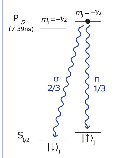
We need to generate photons entangled with our ion qubits in order to implement our ion-photon network.  $\downarrow$ We do this by exciting a <sup>88</sup>Sr<sup>+</sup> ion to one of its shortlived  $P_{1/2}$ -states using a picosecond laser. The emitted 422 nm photon is entangled in frequency and polarisation with the resulting Zeeman qubit.
