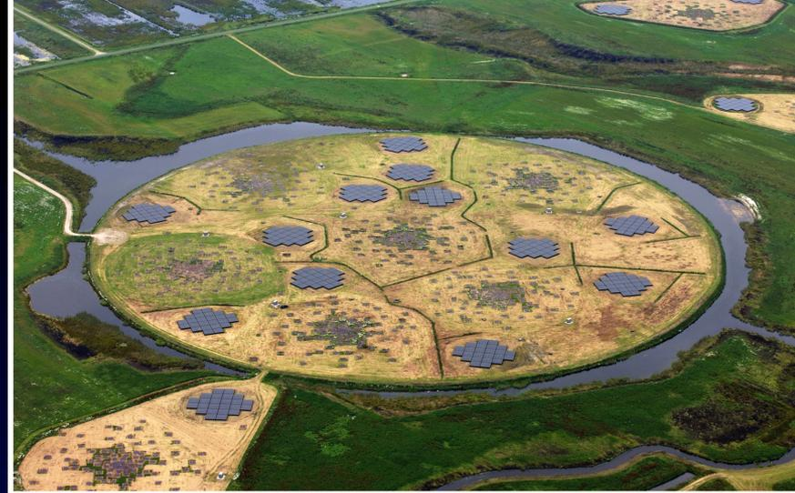
Fig. 1. Aerial photograph of the Superterp, the heart of the LOFAR core, from August 2011. The large circular island encompasses the six core stations that make up the Superterp. Three additional LOFAR core stations are visible in the upper right and lower left of the image. Each of these core stations includes a field of 96 low-band antennas and two sub-stations of 24 high-band antenna tiles each.
