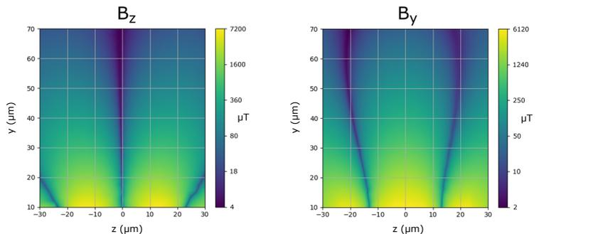
Estimates for field and gradient on RF trap axis for 1 W of microwave power:  $\frac{\partial B_z}{\partial z} = 28 \text{ T m}^{-1}$ ,  $B_y = 300 \mu\text{T}$ ,  $B_z = 6 \mu\text{T}$
