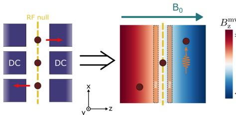
Ions first displaced from RF null via DC field, microwave pulses are then resonant only with desired ion [8]; see also [9] for a different method of addressing
