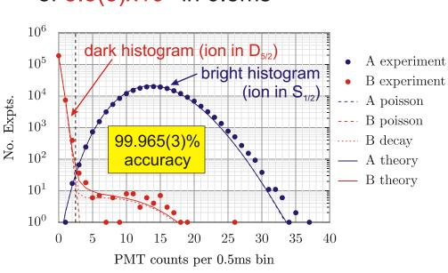
modest increase in net detection efficiency from 0.1% to 0.5% would reduce error to 0.6x10<sup>-4</sup> in 120μs
