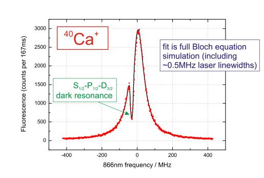
For <sup>43</sup>Ca<sup>+</sup>, it appears difficult to find experimental parameters which give fluorescence rates more than ~30% that of <sup>40</sup>Ca<sup>+</sup>. Efficient repumping from D<sub>3/2</sub> requires large 866nm laser power; however, this gives rise to significant heating effects due to dark resonances which at high power are very broad.
