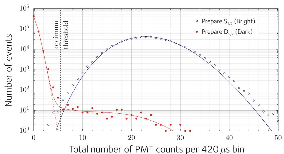
Here the total detection time  $t_b = 420 \,\mu\text{s}$ ; this choice, with a threshold at 5.5 counts, optimizes the discrimination between the bright and dark histograms.
