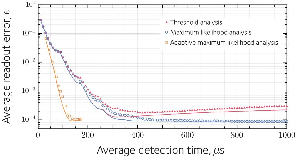
The Maximum likelihood method does not require a precise choice of parameters (threshold and detection time) which must be determined from control data; we only need to know the independently measured rates  $R_B$  and  $R_D$ , and to choose a sufficiently long detection time.
