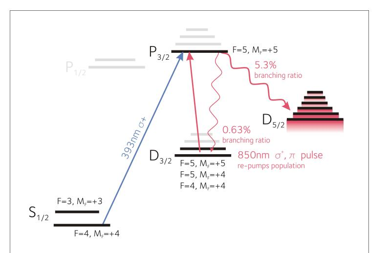
Experiment achieves 99.77(3)% net readout fidelity. Correcting for finite "optical qubit" error [see left], in this case  $1.0(2)x10^{-3}$ , implies transfer fidelity was 99.87(4)%.
