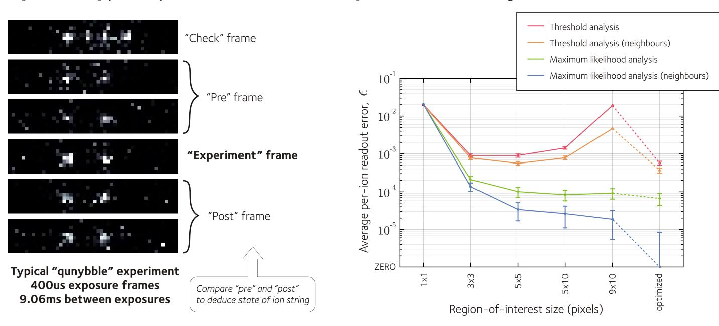
**Threshold** Compare *total summed counts* for all pixels in the region of interest to the threshold value. Above threshold is 'bright' and below threshold is 'dark.'
