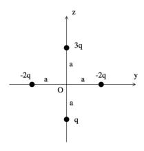
Four charges are placed as shown. Calculate the electric dipole moment of the distribution and find an approximate formula for the potential, valid far from the origin (use spherical coordinates).
