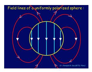
Note that the parallel component of **E** at the surface,  $E_{\theta}(R)$ , is continuous, whereas the perpendicular component,  $E_r(R)$ , is discontinuous:
