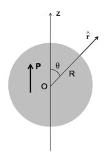
Inside the sphere, the volume charge density is  $\rho_p = -\nabla \cdot \mathbf{P}$ which is 0 as the polarization is uniform. At the surface of the sphere, there is a surface charge density  $\sigma_p = \mathbf{P} \cdot \hat{\mathbf{r}}$ , where  $\hat{\mathbf{r}}$  is the unit vector in the radial direction. We choose the z-axis in the direction of  $\mathbf{P}$ , so that  $\sigma_p = P \cos \theta$  in spherical coordinates.
