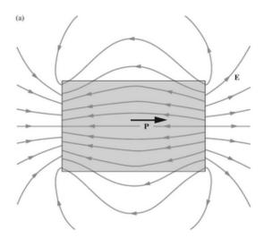
**Electric field**: The bar is therefore like a physical dipole. Note that electric field lines terminate on charges, whether they are bound or free, with **E** pointing towards the negative charge. (Figure from *Purcell.*) The perpendicular component of  $\mathbf{E}$  is discontinuous at the surfaces:
