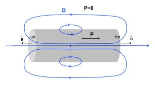
We see that even though there is **no polarization outside** the cylinder, **D** is **non zero** there. This is because the polarization is discontinuous at the surface of the cylinder, and along the lateral surface we have (see equation [2.22] from the lecture notes):
