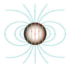
Field lines of a uniformly magnetized sphere. Note that the perpendicular component of **B** at the surface,  $B_r(R)$ , is continuous, whereas the parallel component,  $B_{\theta}(R)$ , is discontinuous:
