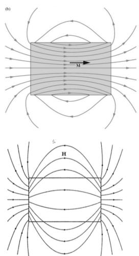
**Magnetic field**: The bar is like a finite–size solenoid. (Figure from *Purcell.*)
