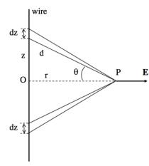
Given the symmetry of the system, the electric field at the point P is:
