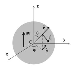
Inside the sphere, the volume current density is  $\mathbf{J}_m = \nabla \times \mathbf{M}$  which is 0 as the magnetization is uniform. At the surface of the sphere, there is a surface current density  $\mathbf{K}_m = \mathbf{M} \times \hat{\mathbf{r}}$ . We choose the z-axis in the direction of  $\mathbf{M}$ , so that  $\mathbf{K}_m = M \sin \theta \hat{\boldsymbol{\varphi}}$  in spherical coordinates.
