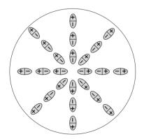
As **P** is radial, the dipoles in the sphere are all aligned in the radial direction, leaving a net charge at the center and at the surface only.
