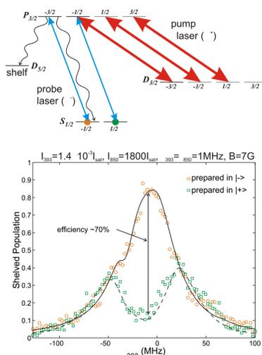
Dip shows suppression of excitation by EIT (unwanted excitation suppressed by factor  $\sim 200$ ; the shelving branching ratio = 5% to give observed ratio shelving/spin relaxation rate  $\sim 10$ ).
