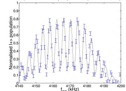
Ramsey fringes as a function of oscillating magnetic field frequency.
