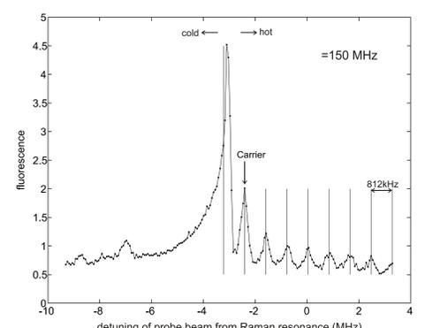
Fluorescence (a.u.) resulting from scanning the probe laser over the Raman resonance.
