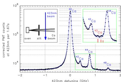
The graph shows the 423nm fluorescence scattered from the atomic beam as the 423nm laser frequency is scanned over the resonance of the various isotopes in the beam.
