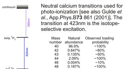
We deduce the cross-section for ionization by the 389nm laser to be 170(60) megabarns.
