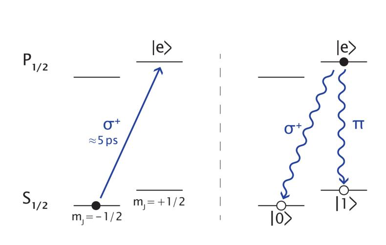
A 88Sr<sup>+</sup> ion is excited to one of its short-lived  $P_{1/2}$ -states using a picosecond laser. The photon emitted in the decay is entangled in frequency and polarisation with the resulting Zeeman qubit.
