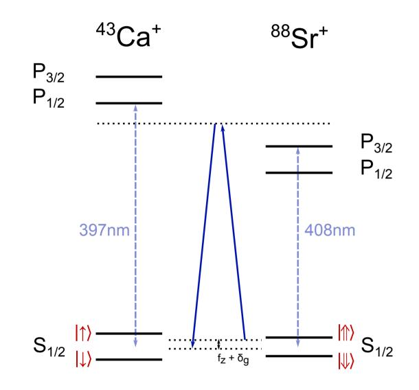
A single pair of Raman beams, detuned by approximately 10 THz from the S-P transitions of both 88Sr<sup>+</sup> and 43Ca<sup>+</sup>, provide the force for a gemoetric phase gate [3].
