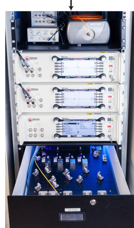
Compact rack-mounted laser systems for 43Ca+ and <sup>88</sup>Sr<sup>+</sup> have been built to house the lasers, optics, AOMs and EOMs necessary for each beam path, with independent control for each of the two trap systems.
