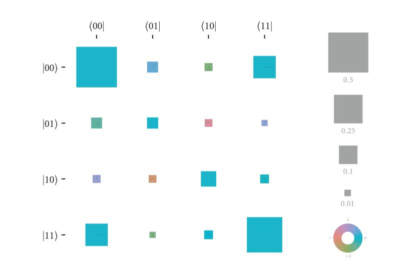
In our initial demonstration, with the emission collected perpendicular to the magnetic field, we obtained a Bell state fidelity of 0.77 (entanglement of formation 0.081).
