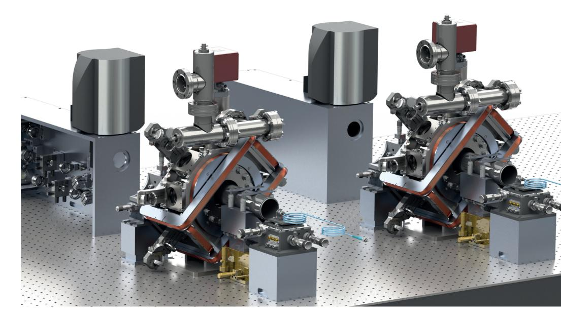
Two identical vacuum system assemblies, each containing a HOA2 linear multi-zone surface trap (courtesy of Sandia Nat'l Labs), are currently under construction.
