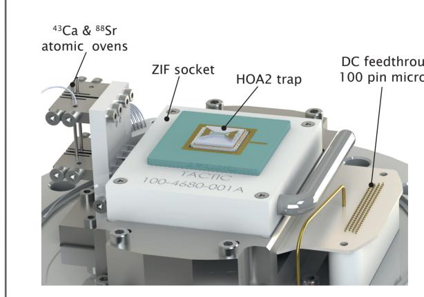
As the time between recrystallisation events may limit experiments, we have designed atomic ovens optimised for short loading times, by reducing their thermal mass and controlling the oven temperature.
