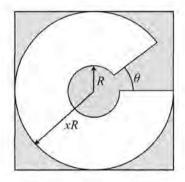
(a) Area of C-shape Ac is a fraction of the difference of the areas of the outer and inner circles proportional to the fractional angle covered by the C-shape.
