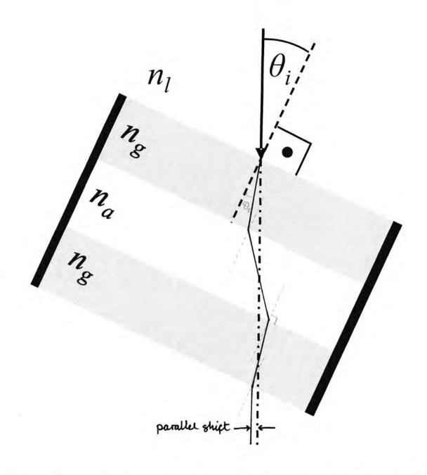
(a) The angles at the glass-air and air-glass interfaces are bigger than those at the liquid-air and air-liquid interfaces.
